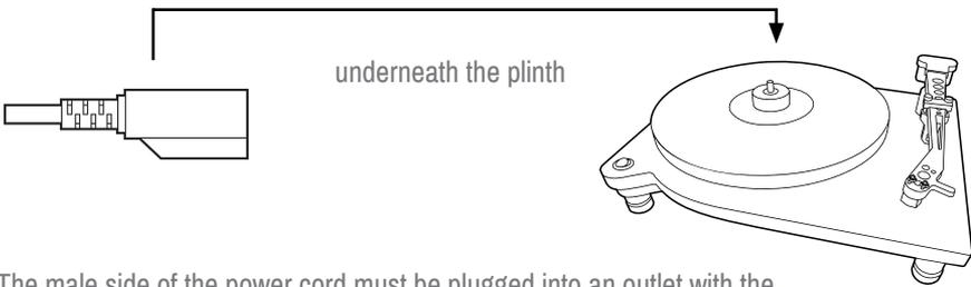
The male side of the power cord must be plugged into an outlet with the cord facing downwards.
